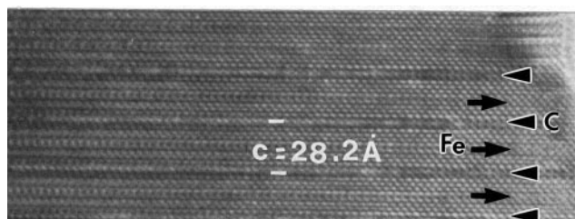
Fig. 4 [100] HREM image showing the local stabilization of the member [\text{Sr}_4\text{Fe}_3\text{O}_{10}]_1 [\text{Sr}_4\text{Fe}_2(\text{CO}_3)\text{O}_6]_1 .
